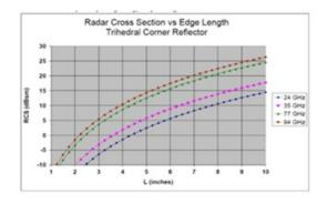
**Radar cross section (RCS)**: is the measure of a target's ability to reflect radar signals in the direction of the radar receiver, i.e. it is a measure of the ratio of backscatter power per steradian (unit solid angle) in the direction of the radar (from the target) to the power density that is intercepted by the target.
