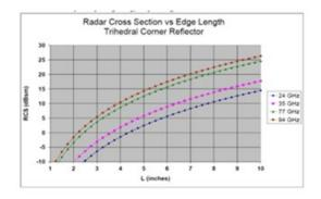
**Radar cross section (RCS)**: is the measure of a target's ability to reflect radar signals in the direction of the radar receiver, i.e. it is a measure of the ratio of backscatter power per steradian (unit solid angle) in the direction of the radar (from the target) to the power density that is intercepted by the target.
